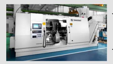
Machining components measuring up to 450 mm in diameter and 1500 mm in length, used to turn the ends and supports of the various crankshafts
